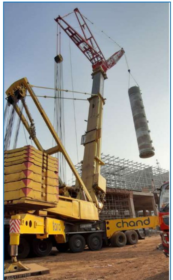
Unique Lifting Solutions for Steel, Cement, Oil & Gas, Power, Chemical, Renewable Energy Sectors (Crane in the pic is Liebherr LTM 1800 800MT Capacity)
