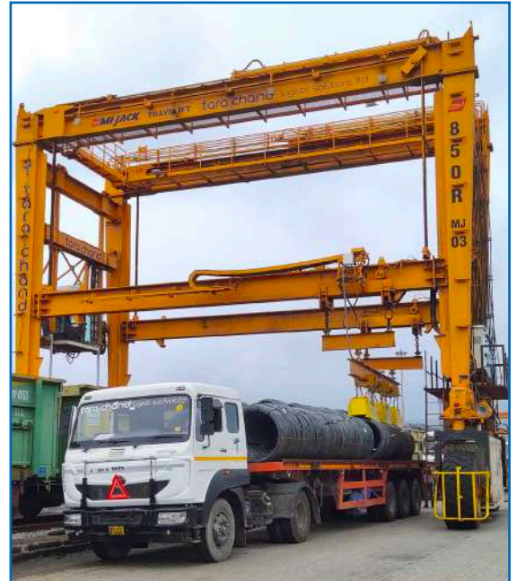
Mi-Jack Rubber Tyre Gantry Crane at the Central Dispatch Yard, RINL, Visakhapatnam.
